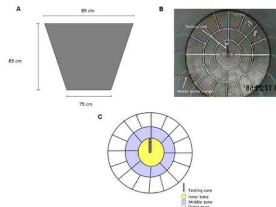
**Figure 1.** The circular open field, an aluminum tub-shaped apparatus with a based-diameter of 75 cm, an opening-diameter of 85 cm with a height of 85 cm (A). The water bottle hanger and a metal testing core are installed for water dispensing during 24-hour test and for cardboard paper placer, respectively (B). The base of the apparatus was divided into 3 zones; inner zone, middle zone and outer zones as shown in C.
